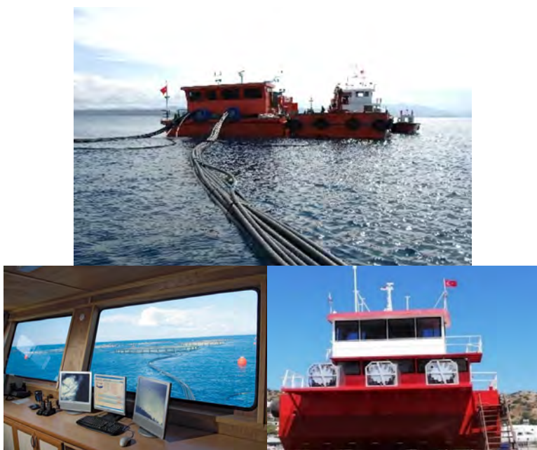
Figure 8. Automatic feeding barge system and feeding system management room (DGFA 2020b)
